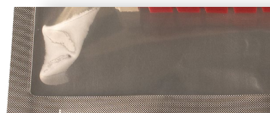
+ Above and below - examples of the broad textured seal produced by the Shawseal.
